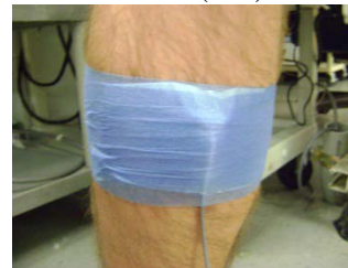
Picture 6: Pre-wrap over tape and electrode for extra adherence
