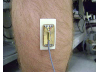
Picture 4: Electrode attached to prepped site (GN)
