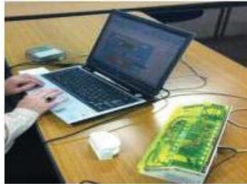
Every IC Tag card can be connected with Powerpoint slides (one IC Tag for one slide). All information is saved in an Access database. Every time that IC Tag card touch IC Tag reader (see Fig. 5), the slide connected with this card is displayed on computer screen (except computer screen also video projector can be used).
