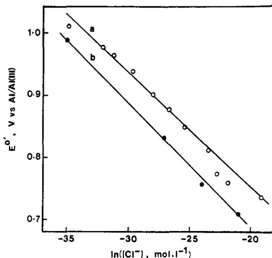
**Figure 5.** Plots of  $E^{\circ'}$  vs.  $\ln [\text{Cl}^-]$  for the Sb(III)/Sb couple in acidic melts: a, from potentiometry; b, from voltammograms of Sb(III) solutions on RGCDE obtained from a reverse scan (see text).
