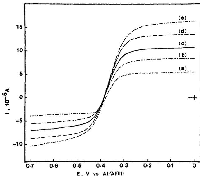
Figure 11. Voltammograms of a solution of Sb(III) and Sb(V) in 0.75:1 melt, at RGCDE ( $[\text{Sb(III)}] = 10.2 \times 10^{-3} \text{ M}$ ;  $[\text{Sb(V)}] = 10.2 \times 10^{-3} \text{ M}$ ). Rotation rate/rpm: a, 400; b, 900; c, 1600; d, 2500; e, 3600.
