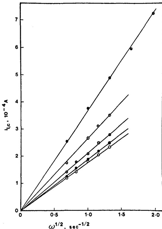
**Figure 3.** Limiting cathodic currents for the reduction of Sb(III) vs.  $\omega^{1/2}$ :  $\otimes$ ,  $8.2 \times 10^{-3}$  M in 2:1 melt;  $\circ$ ,  $7.0 \times 10^{-3}$  M in 1.5:1 melt;  $\ominus$ ,  $6.2 \times 10^{-3}$  M in 1.24:1 melt;  $\bullet$ ,  $5.7 \times 10^{-3}$  M in 1.09:1 melt;  $\circ$ ,  $5.5 \times 10^{-3}$  M in 1.01:1 melt.
