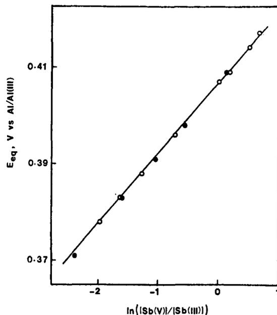
Figure 9. Potentiometric data for the Sb(V)/Sb(III) couple in the 0.75:1 melt.
