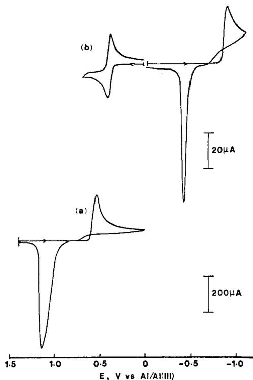
**Figure 1.** Cyclic voltammograms of Sb(III) melt solutions: a,  $7.0 \times 10^{-3}$  M in 1.5:1 melt,  $\nu = 20 \text{ mV s}^{-1}$ ; b,  $6.3 \times 10^{-3}$  M in 0.8:1 melt,  $\nu = 5 \text{ mV s}^{-1}$ .
