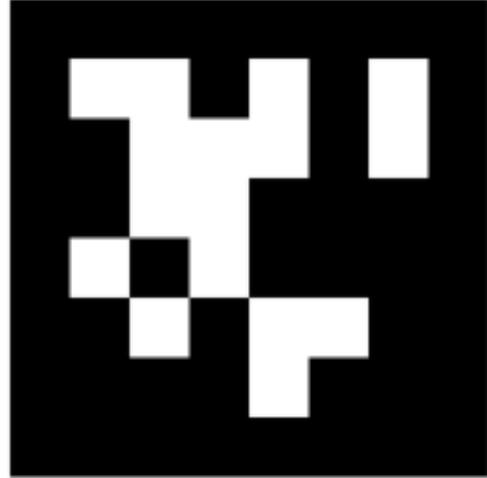
Fig. 1 Above displays an example of an April Tag family 36h11 tag 0
