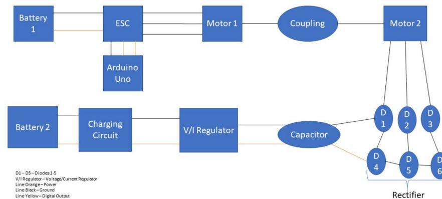
Fig. 3 - Physical form of the Energy Regeneration System
