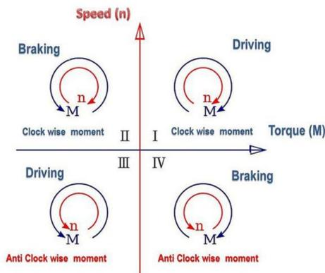
Fig. 1: Regenerative Braking Chart
