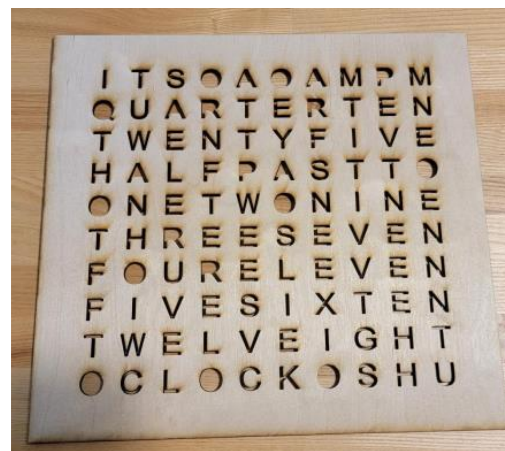
Figure 1: A laser cutter was used to create the face plate for the clock
