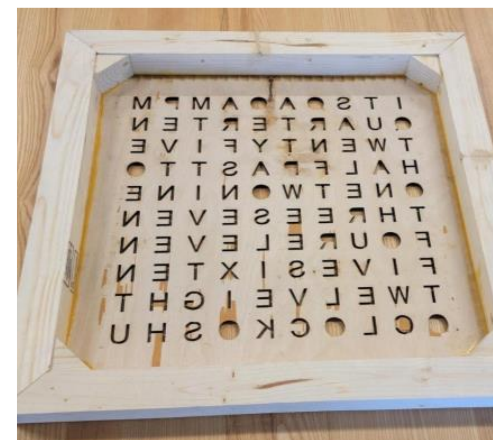
Figure 2: A 2x4 was used to assemble the outer bezel of the frame
