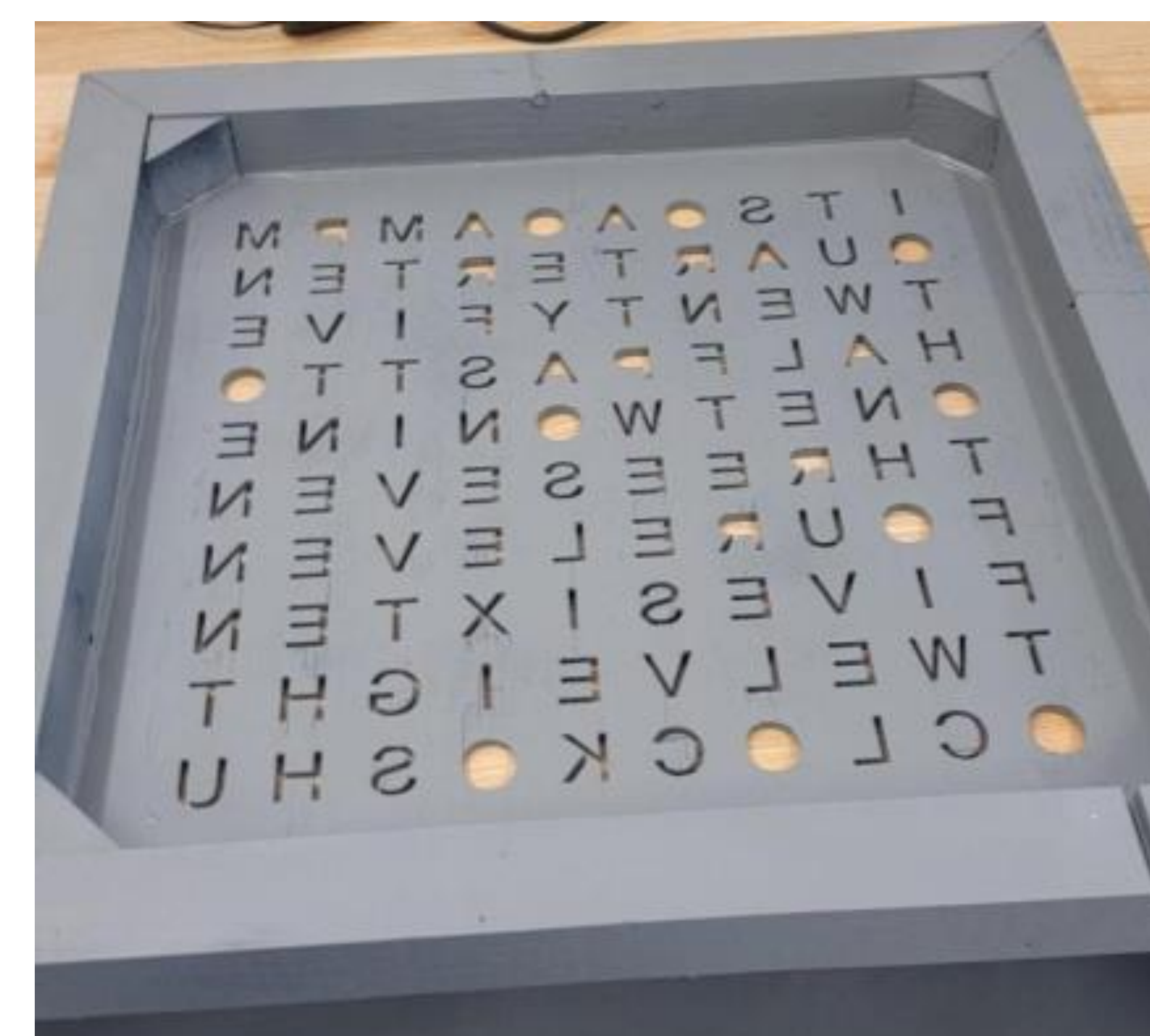
Figure 3: The bezel was primed and spray painted
